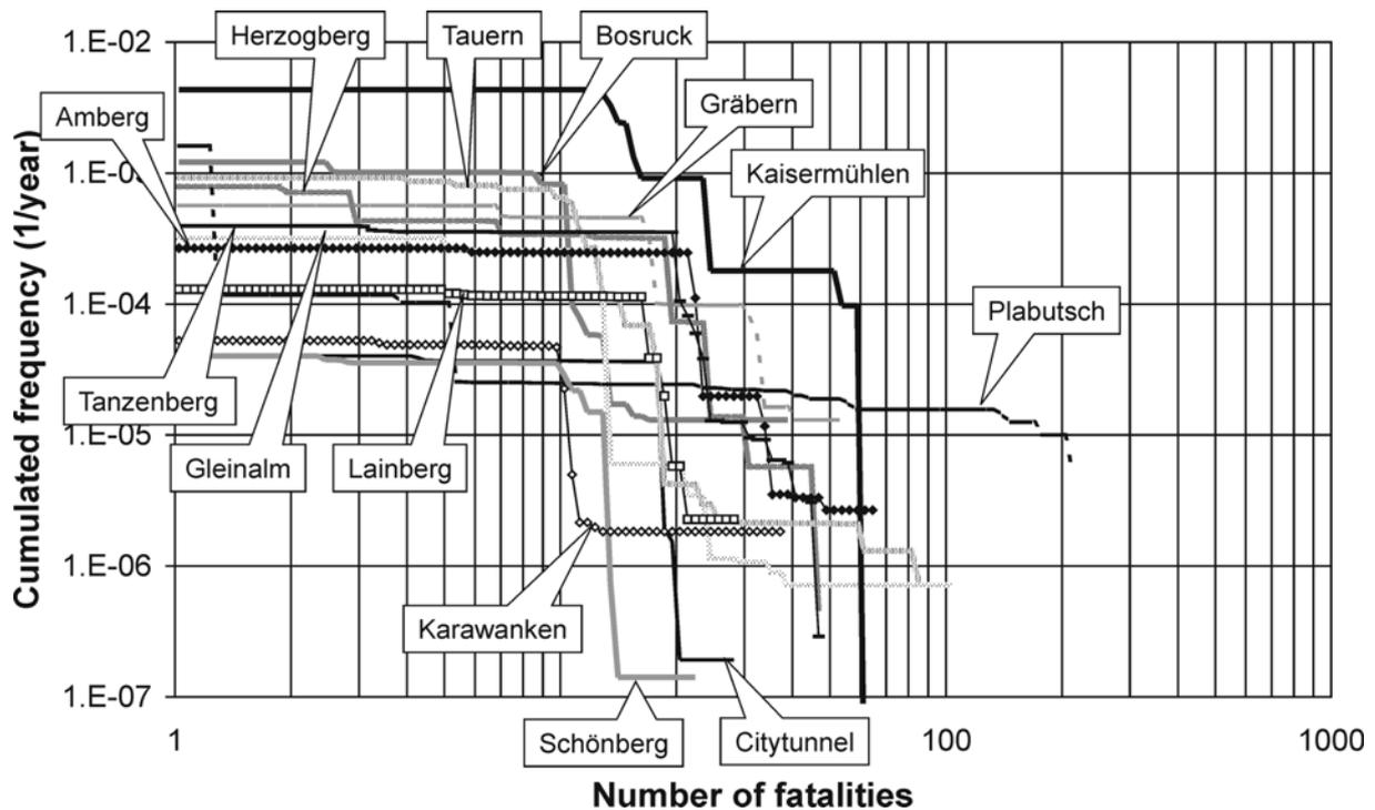
Figure 3: Comparison of the F/N curves of the 13 case study tunnels
