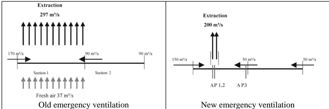
Figure 6: Ventilation systems Bosrucktunnel
