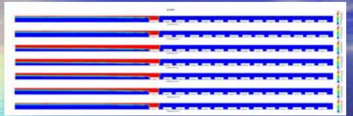
隧道进口段50MW火灾模拟(单向行车; 纵向通风+半横向排烟) 之烟雾浓度扩散分布 Smoke concentration field fire location: near to entrance HRR: 50MW traffic mode: unidirection ventilation mode: longitudinal and semi-transverse
