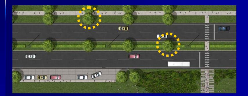
Obstacles located within the clear-zone distance must be removed, relocated, redesigned or shielded by traffic barriers
