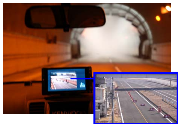
Photo 1. Providing Information by Storing then Reproducing Still Pictures (Warning of a Closed Lane Beyond a Tunnel Exit)
