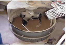
A mixing time of 30 seconds is generally used in the laboratory, which is longer than in situ mixing. Due to the lack of appropriate laboratory mixers in South Africa, CSIR Transportek is designing and manufacturing a new type of mixer, shown below, to enable better simulation of field conditions.
