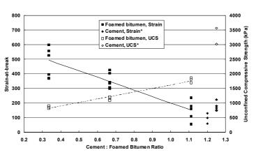
the material (UCS) will increase by adding active filler but flexibility will decrease (see the graph). Flexibility will increase by adding bitumen but then the strength may decrease. It is very important to find the optimum active filler to bitumen ratio for each specific design.
