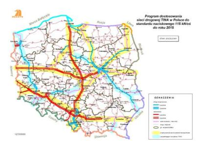
Fig. 9. Program of upgrading main Polish road network to EU standard load 115 kN by 2015
