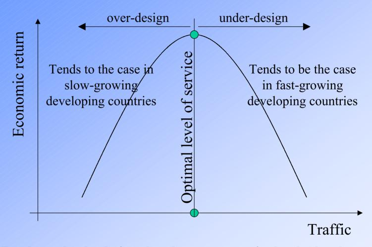
Roads need to be designed to the correct service level related to traffic and then gradually adjusted with growing traffic
