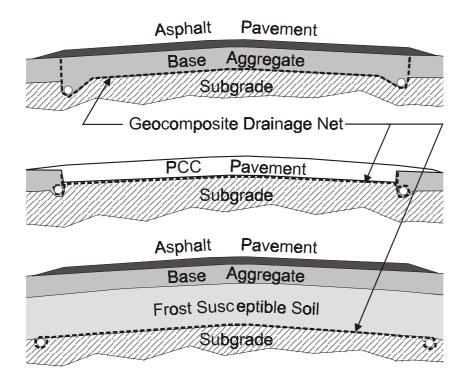
Figure 2. Potential applications of geocomposite drainage net.
