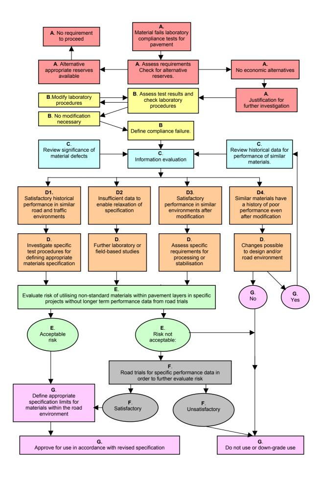
Figure 2 Evaluation of non-standard materials for use in pavements
