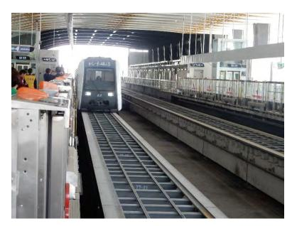
With electromagnetic force, the trains will be suspended above tracks about 10 mm, thus avoiding friction noise between wheels and rails and causing very little vibration.
