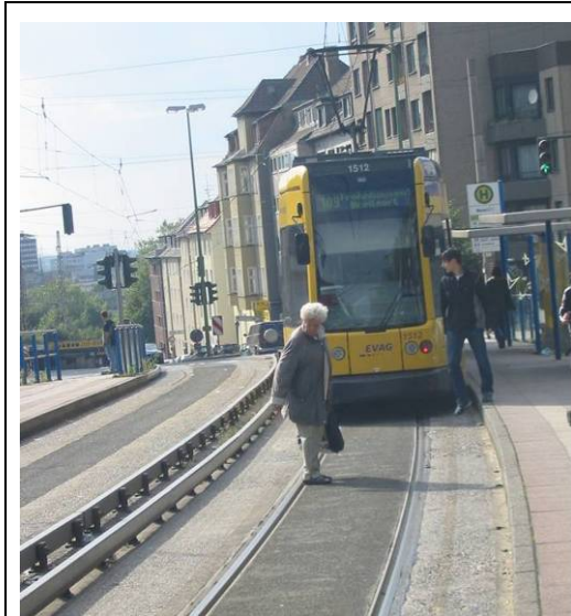
g) Combined running with trams, Essen O-Bahn, Germany
