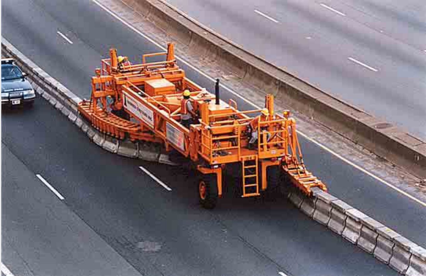
Moveable Construction Barrier
