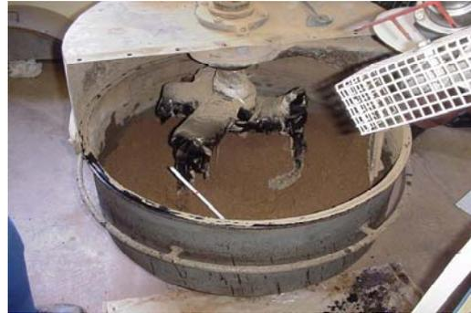
A mixing time of 30 seconds is generally used in the laboratory, which is longer than in situ mixing. Due to the lack of appropriate laboratory mixers in South Africa, CSIR Transportek is designing and manufacturing a new type of mixer, shown below, to enable better simulation of field conditions.
