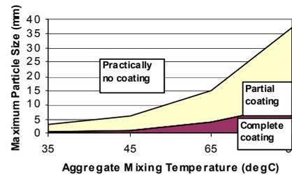
Laboratory mixes should be produced at temperatures similar to that expected during field recycling. It is suggested that recycling with foamed bitumen should not take place when the aggregate temperature is lower than 10°C. The quality of the foamed bitumen can compensate for low aggregate temperatures within certain limits, as shown in the table. The foam index is a measure of the combined expansion ratio and half-life.
