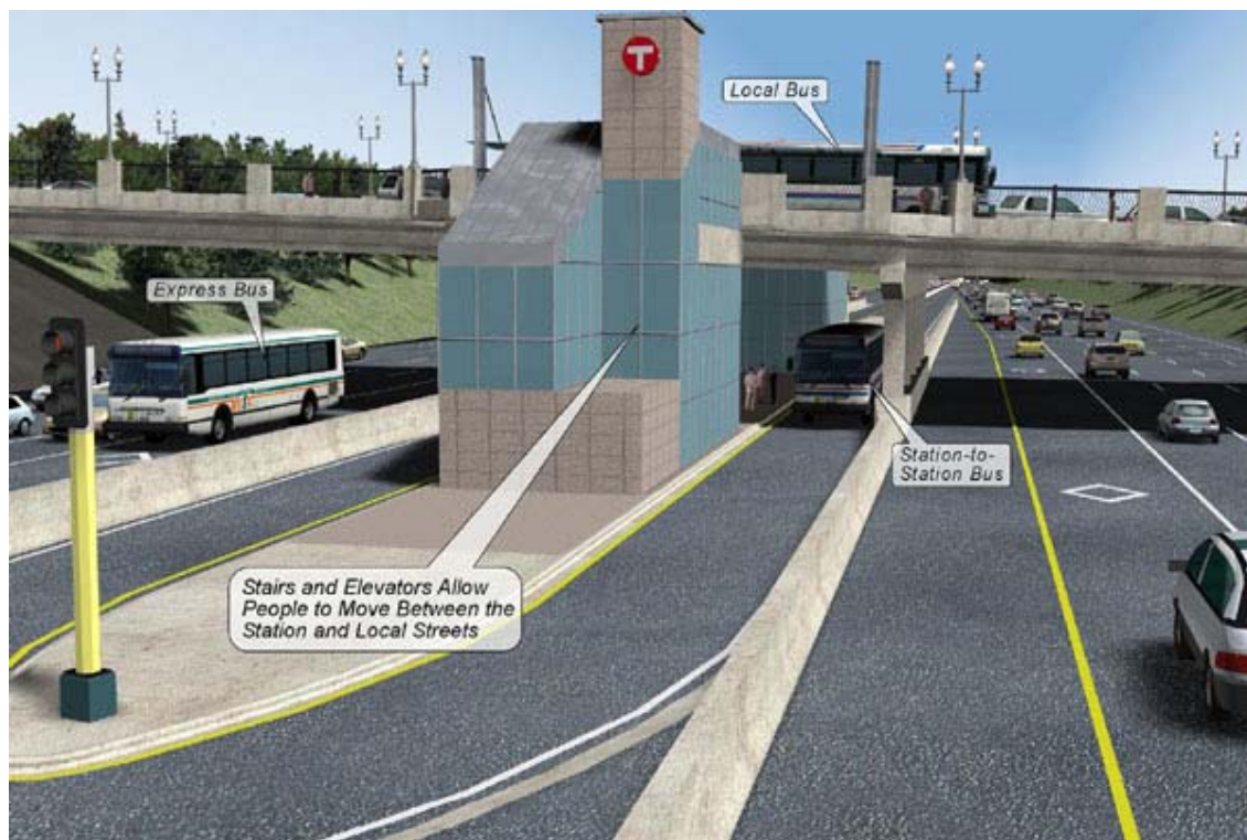
Figure 6B: Possible Concept for an In-Line Toll Managed Lane Bus Rapid Transit Station (Courtesy of Minnesota Department of Transportation, I-35W Project, 2004)
