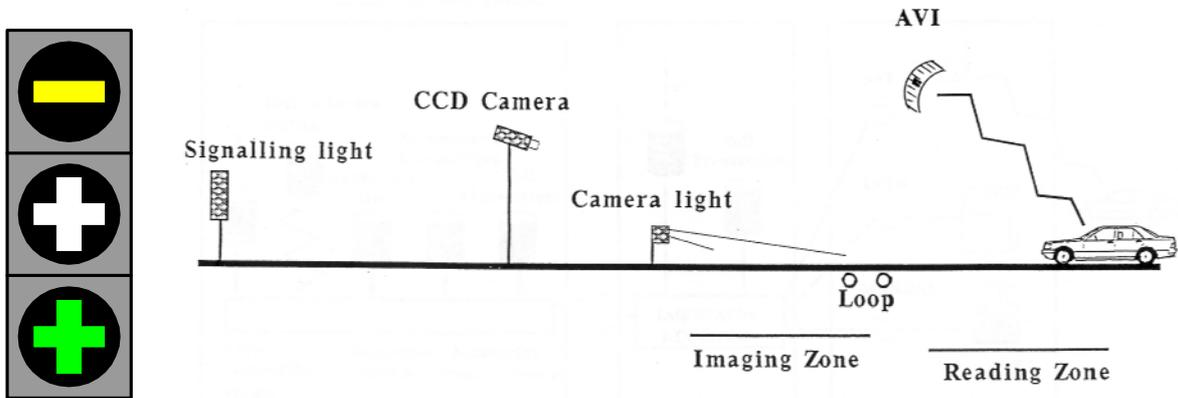
*Figure 6: The equipment in a Norwegian EFC lane*
