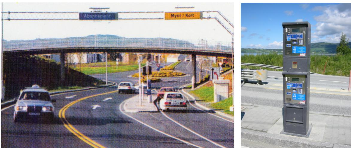
*Figure 7: An unmanned toll plaza in Trondheim with a two level low cost coin machine*
