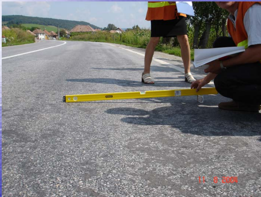
Negative crossfall in the curve
